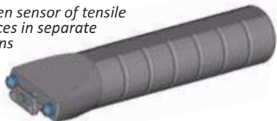
Closed sensor of tensile forces in separate yarns
