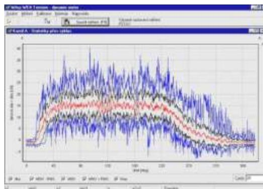
Calculation of statistics from selectable number of machine's periods. (red mean value of tension force, black mean value standard deviation, blue minimum and maximum values of tension force)
