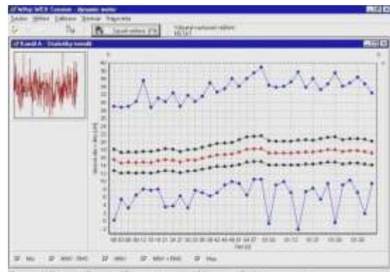
Time development of non-periodical tension force represented by mean value, mean value standard deviation, maximum and minimum values. This measurement is suitable for measuring of long-term trends of tension force.
