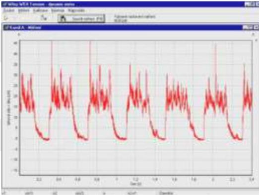
Measurement of non-periodical tension force time waveform.
